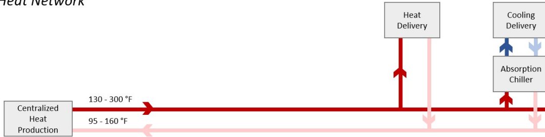
Figure 2: Schematic view of three thermal networks: heat, cooling, and tempered water networks 18
